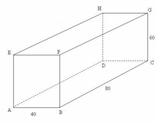
The longest road which can fit into the box will have one end at A and other end at G (or any other similar diagonal)
